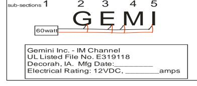
Apply manufacturer label to power supply (first Section)
